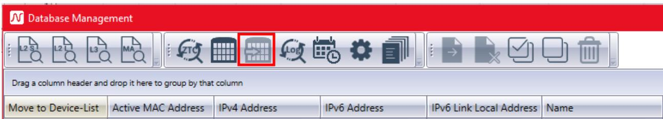
By using this feature, the controller will read the configurations of every selected device and saves them as 'IP\_Address.cfg'. Afterwards, the Devices will be added to the Predefined Devices List selecting the corresponding configuration.
