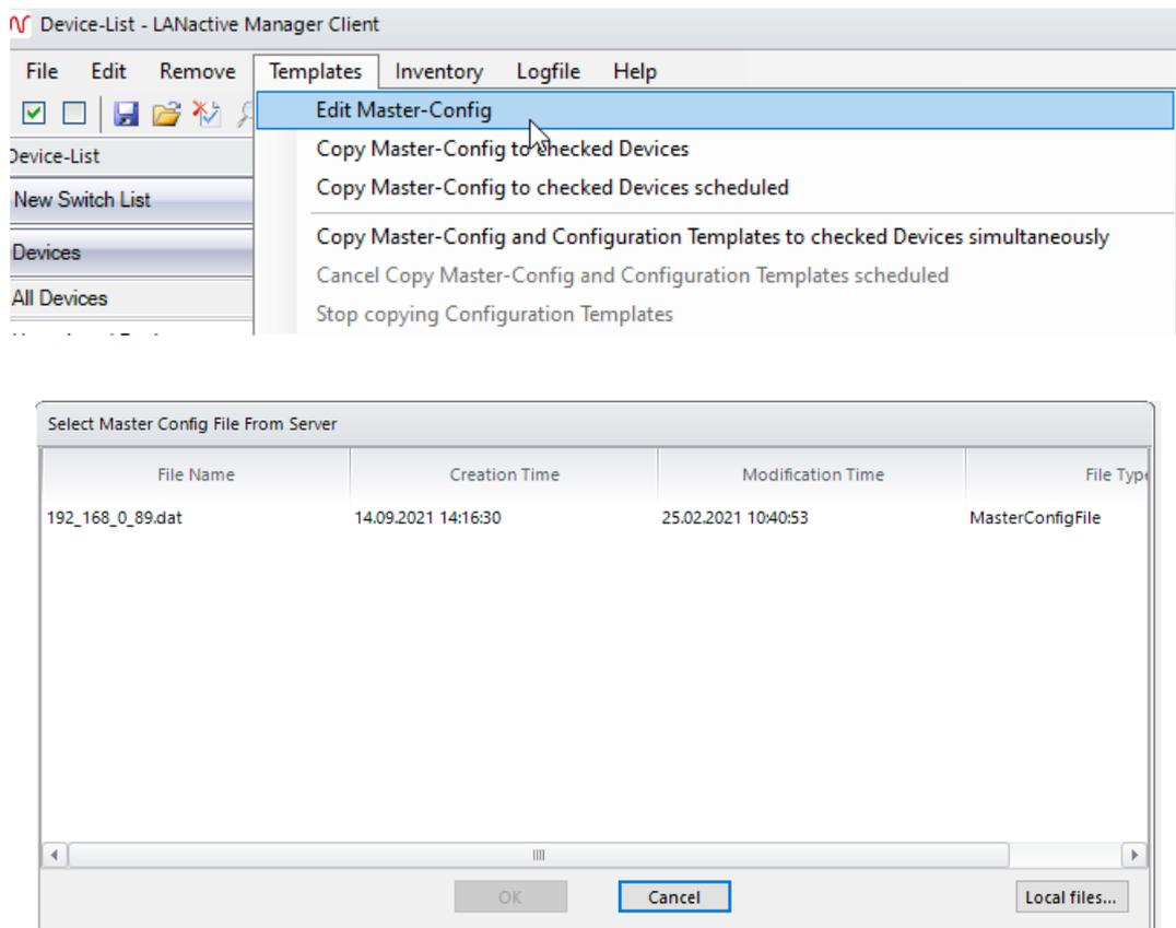
After finished editing, the changes will be saved locally. The file must be uploaded to the controller to be able to send it to any Device. This can be done by clicking “**Save & Upload**” or answering the question whether the file should be uploaded with ‘yes’ after clicking “**Exit & Save**”.
