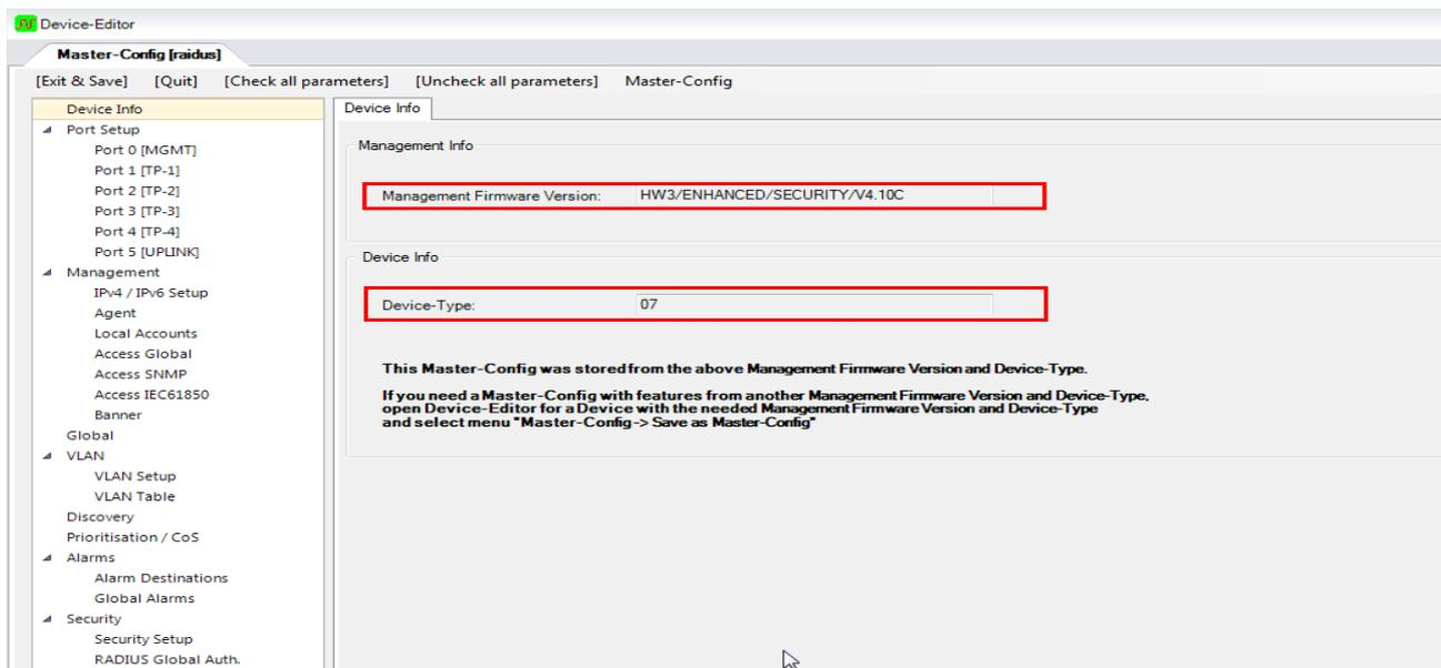
This message reminds you that the master configuration was created for a particular device type (in this example for Device Type 34; the respective device type is indicated on the Info tab).
