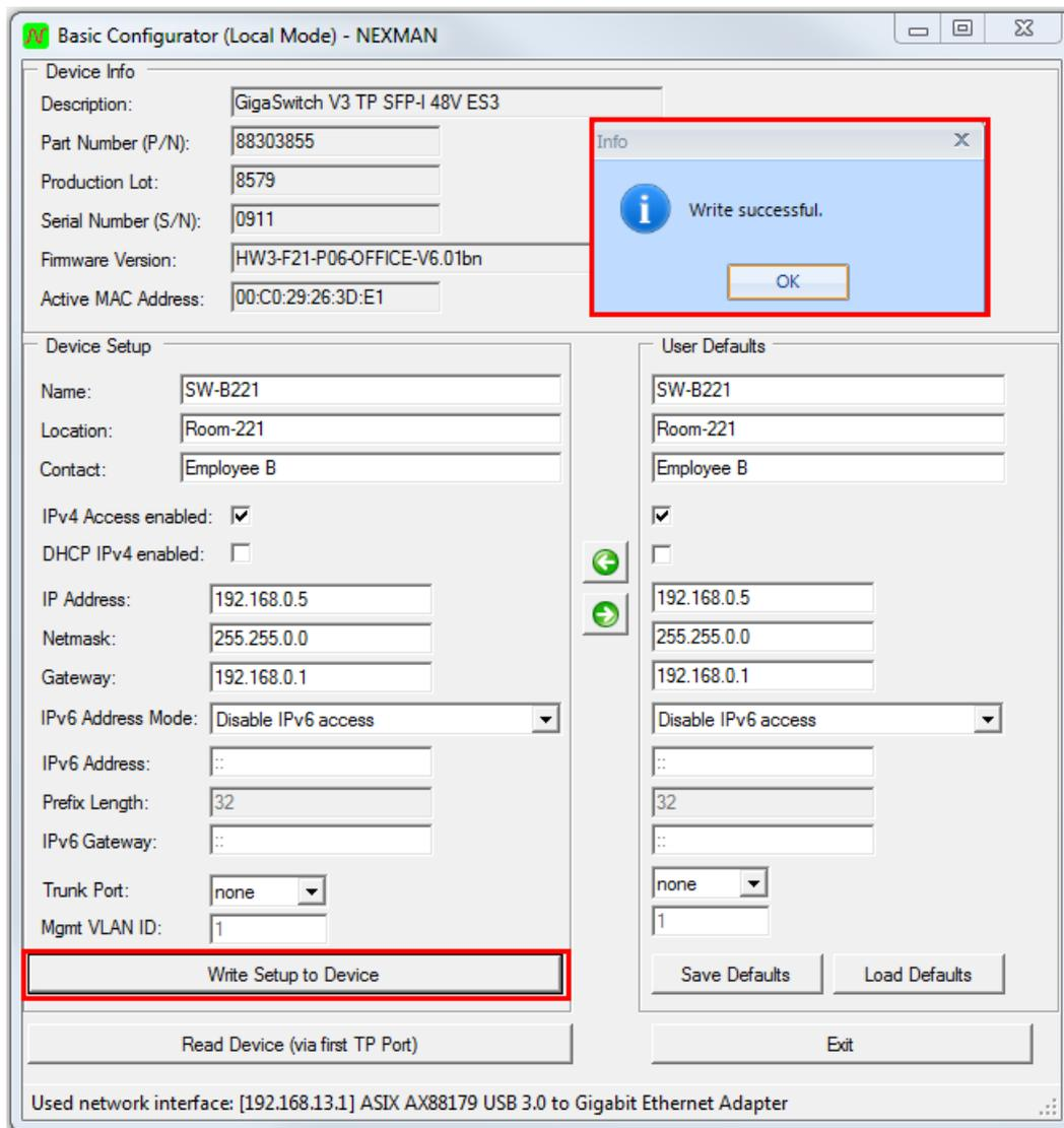
A message in the left lower corner informs about the successful completion of the write operation.
