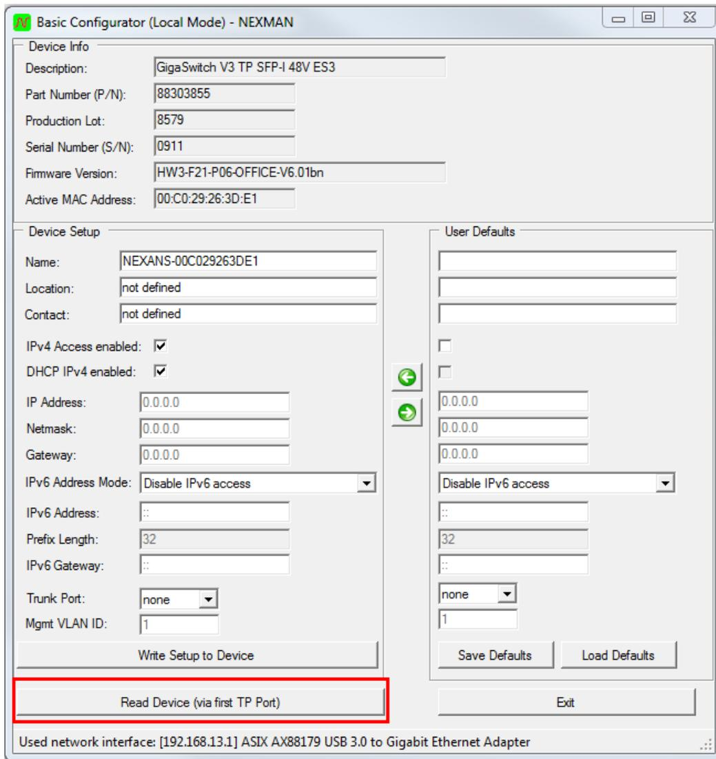
If the configuration has been correctly read, the respective values will be displayed in the **Device Info** and **Device Setup** fields and can be modified. The data in the **Device Info** window is Read-Only and meant for your information only.
