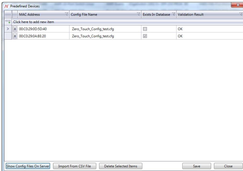
To add multiple MAC Addresses and config files at once, click **'Import From CSV File'**. This file should only contain the MAC Address and the name of the configuration file. If the configuration file is not known to the Controller (not uploaded yet), the corresponding cell remains blank and an error is listed.
