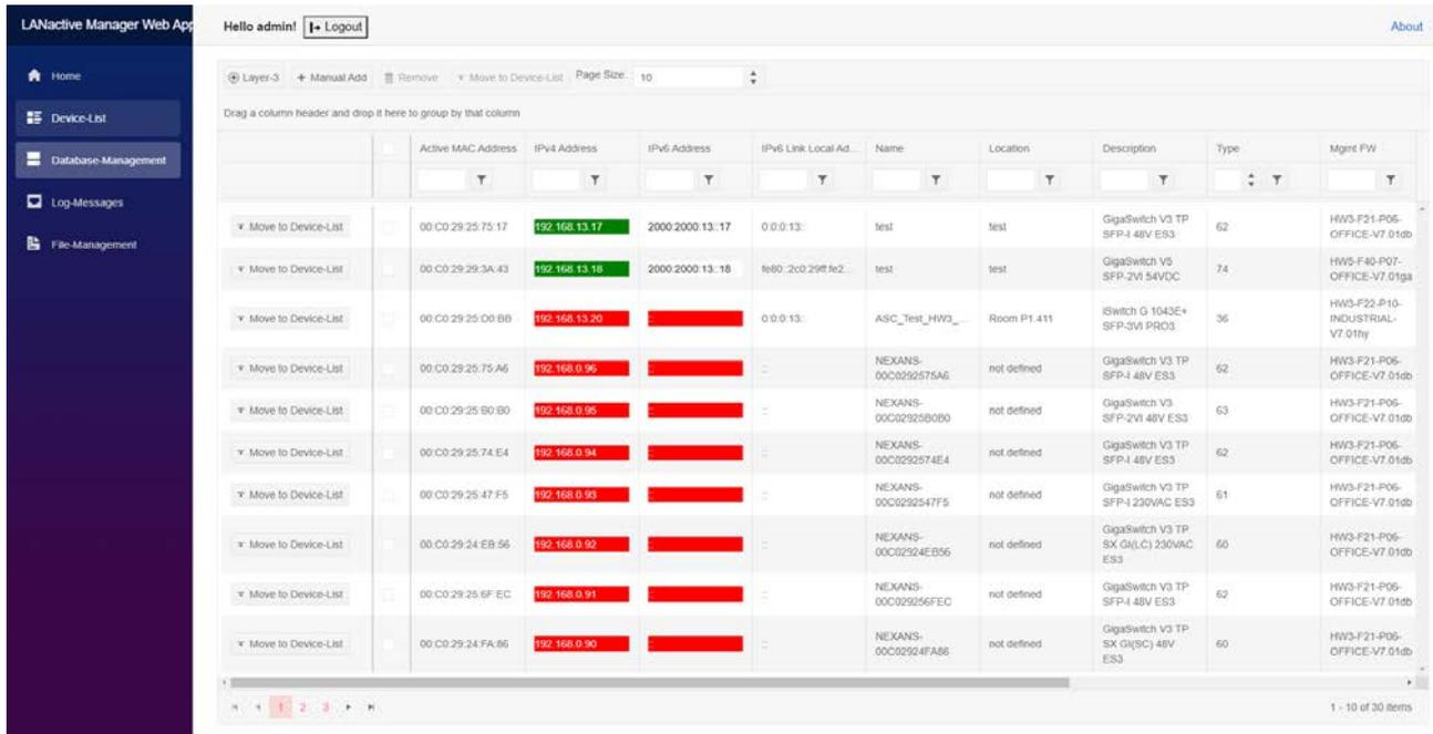
The Database-Management includes functionalities to add Switches by entering a specific IP Address or using Layer 3 Autodiscovery, to add Switches to any Device-List or to remove them from database.
