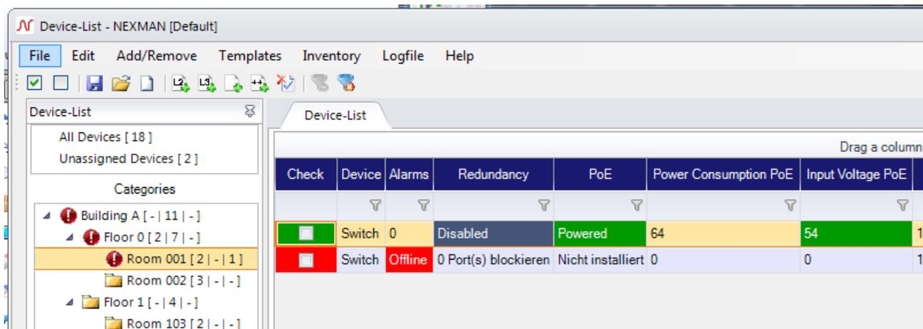
After you have corrected the error the number of errors and the symbol representing it, independently change to its normal state again.
