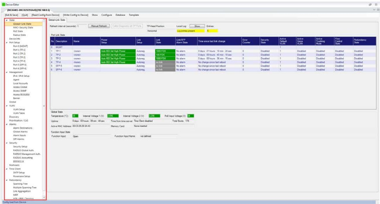
On the state pages (Tabs "Global+Link State", "MAC+Security State" and "PoE State") always the current state of the device is displayed, independent of whether changes have been made in the other tabs (Agent, Access, Global, ...) and not yet transferred into the device.
