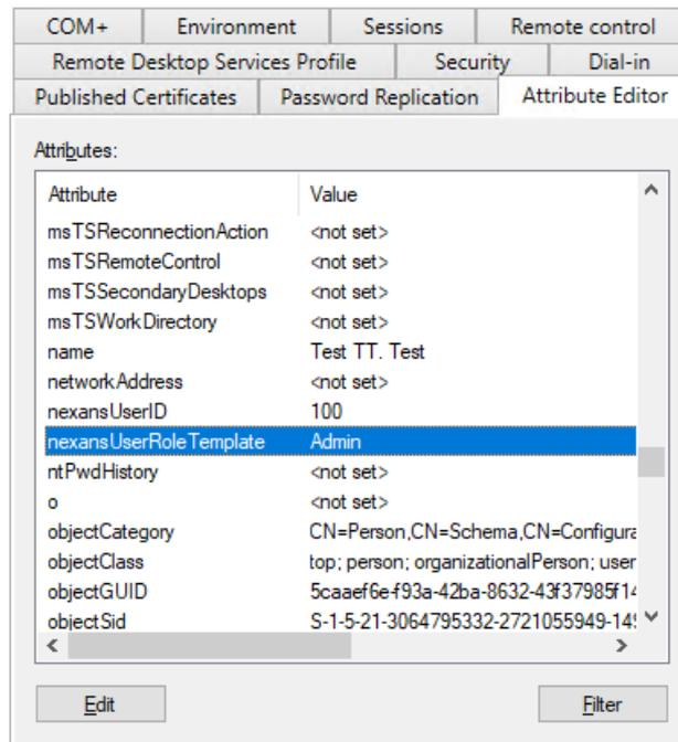
The value of “nexansUserRoleTemplate” must be equal to one of the Role Templates which can be defined in the User Management (see chapter 11.5 *User Management in Client/Controller-Version*).
