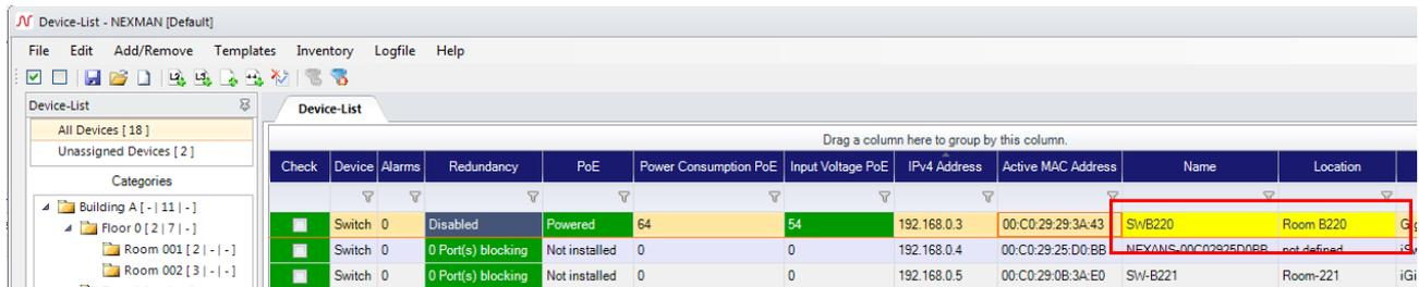
The **Edit > Acknowledge changes of checked Devices** menu can be used to remove the yellow background colour of the fields:
