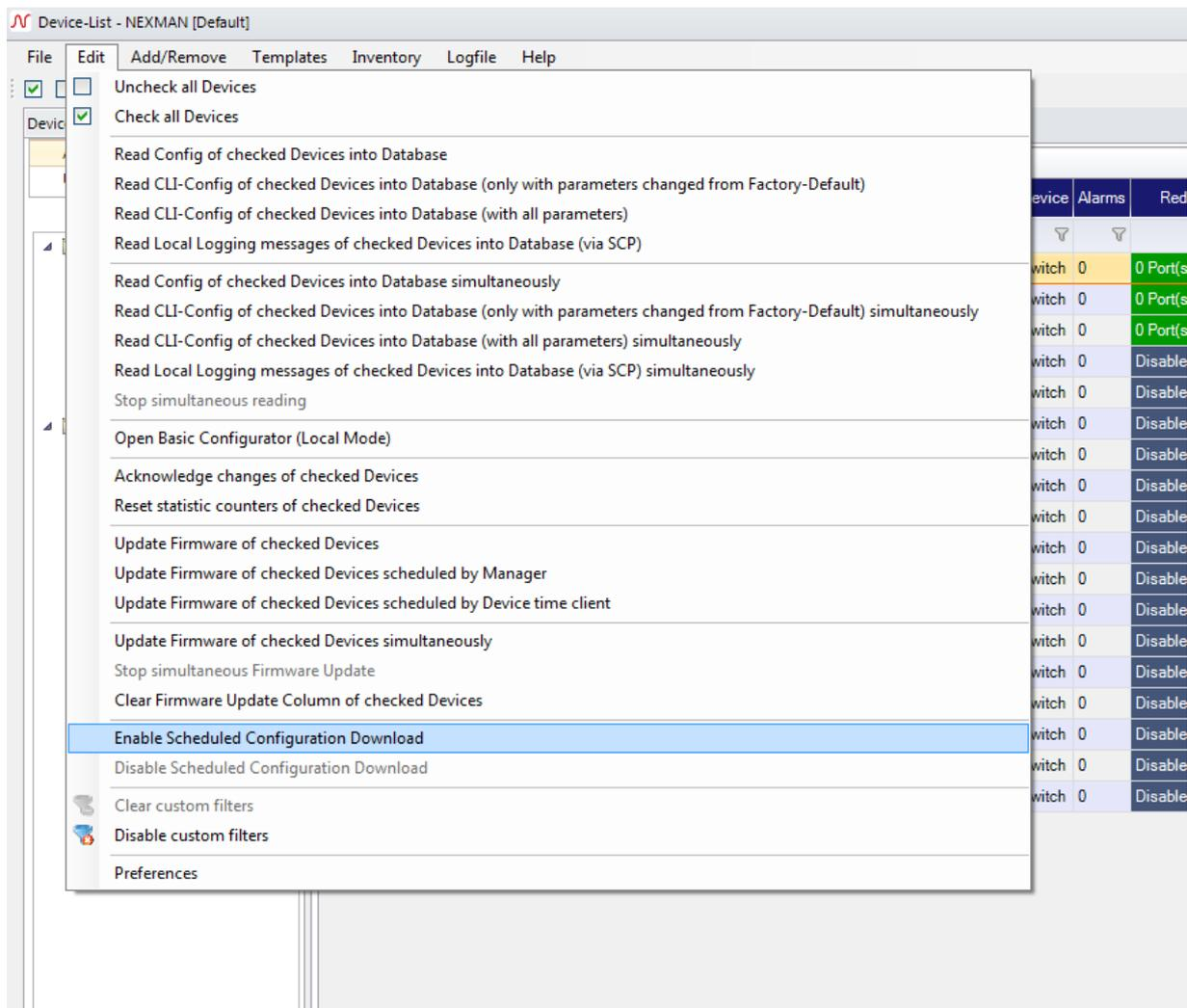
Via **Edit > Enable Scheduled Configuration Download** you can start the process. Afterwards the configuration of each device in the current device list will be read into the database at the given time each day. A notification inside the status bar shows whether the scheduled download is activated or not.
