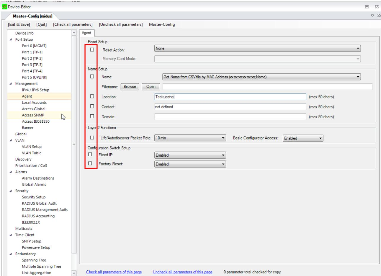
These check boxes allow you to choose which parameters are to be distributed to other devices. No other parameters will be changed in the target devices, i.e. the settings for these parameters are irrelevant as long as the respective box is not checked.
