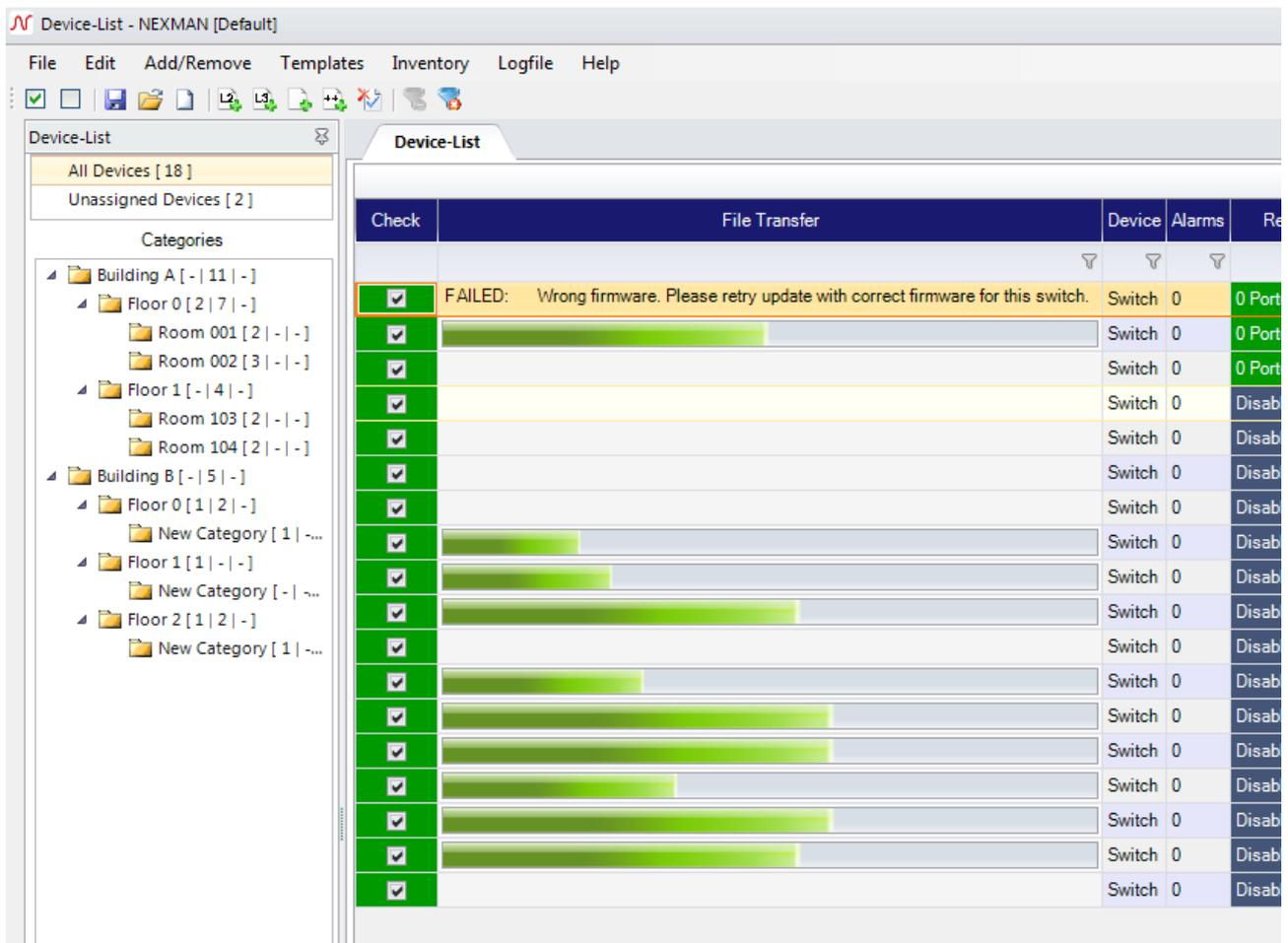
If you have decided to wait until the switch has rebooted, a message is shown while the switch is flashing and rebooting. The flashing process will be also underlined with a blinking check column. While rebooting the switch is marked as "offline".
