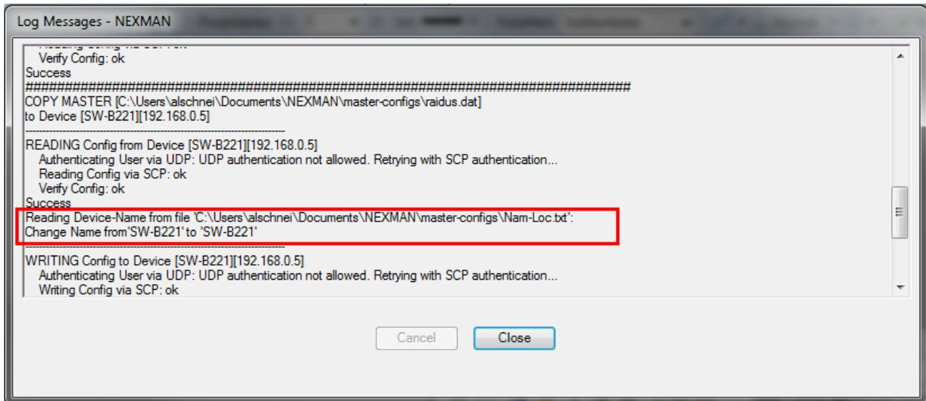
If the respective MAC address is not found in the CSV file, a corresponding error message is returned and the name or location will not be changed. However, all other parameters of the Master configuration, which have been selected by Master check marks, will be accepted:
